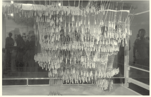
Antonio Gaudi's inverted structural model of hanging chains.
