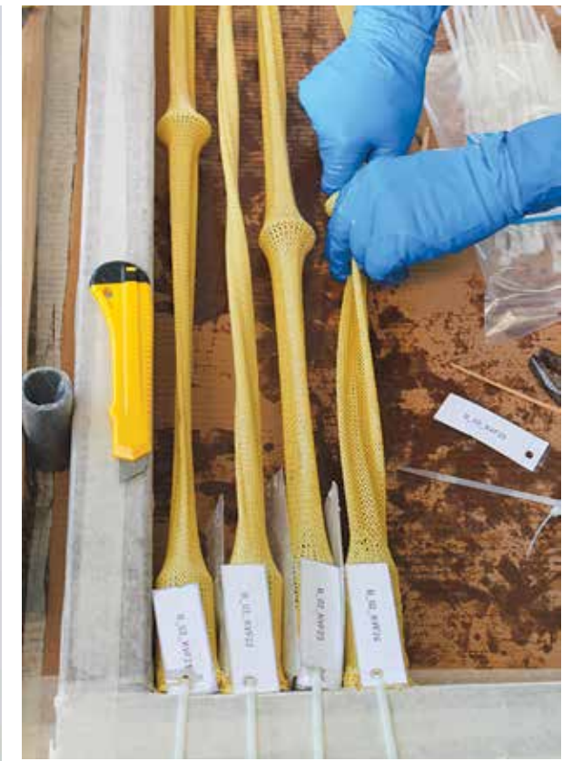
Figure 7 Forming process by fabric manipulation introduces qualities of craft into the industrial setup of composite manufacturing.
