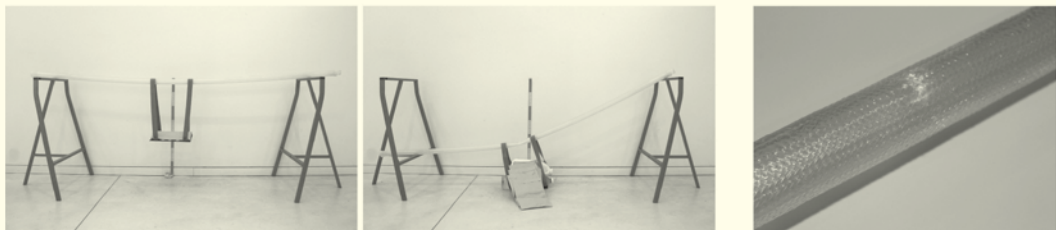
Bending test for fiberglass component.
